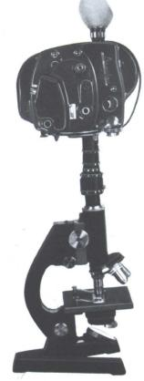
The same set of extension tubes is utilisable for microcinematography, tube size being determined by the desired degree of magnification. They screw directly into the camera (in place of the lens) and are adapted to the microscope ocular by means of a baffle-type adaptor ring. Focusing is performed directly on the ground-glass of the reflexviewing system.
